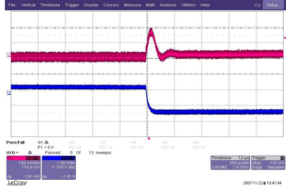
[Fig.6] Load step: 70%-50% of I_o , di/dt=0.1A/\mu s (CH1: 100mV, CH2: 5A/div, 200us/div)
