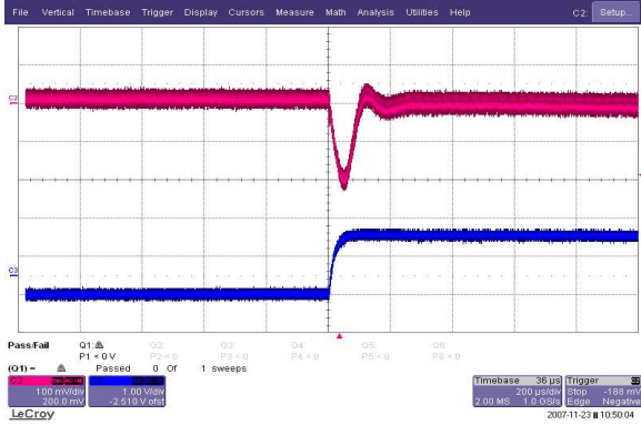
[Fig.5] Load step: 50%-75% of I_o , di/dt=0.1A/\mu s (CH1: 100mV, CH2: 5A/div, 200us/div)
